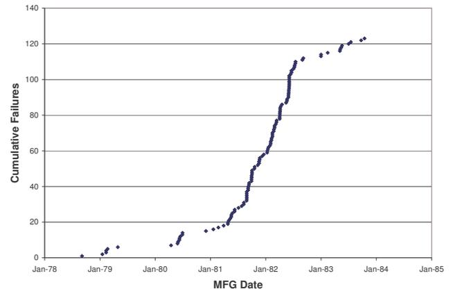
Figure 7: Cumulative failures of 29mm BSCC heart valve based on valve manufacturing date.
