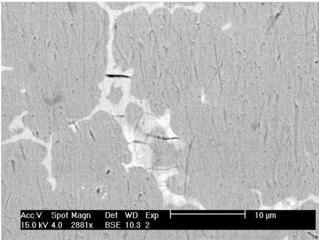
Figure 5: Incipient cracking in inter-dendritic region of weld between outlet strut and valve ring.
