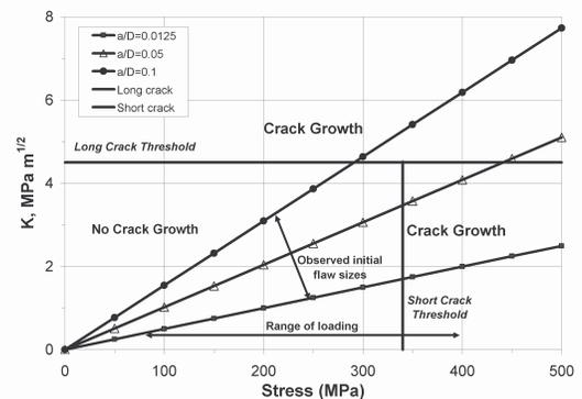
Figure 6: Calculated failure envelope for outlet strut in the BSCC heart valve.
