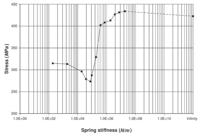
Figure 2: Outlet strut root stress as a function of equivalent aortic stiffness.
