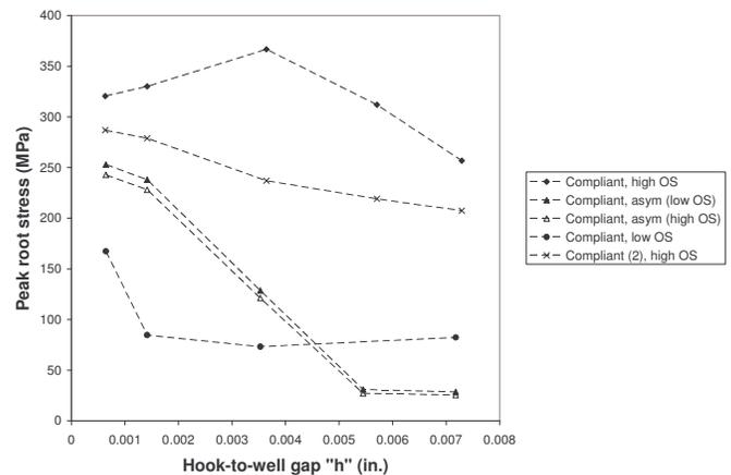
Figure 4: Effect of hook to well gap and position of attachment of outlet strut legs to valve ring on stresses at root of outlet strut for a valve with compliant support.
