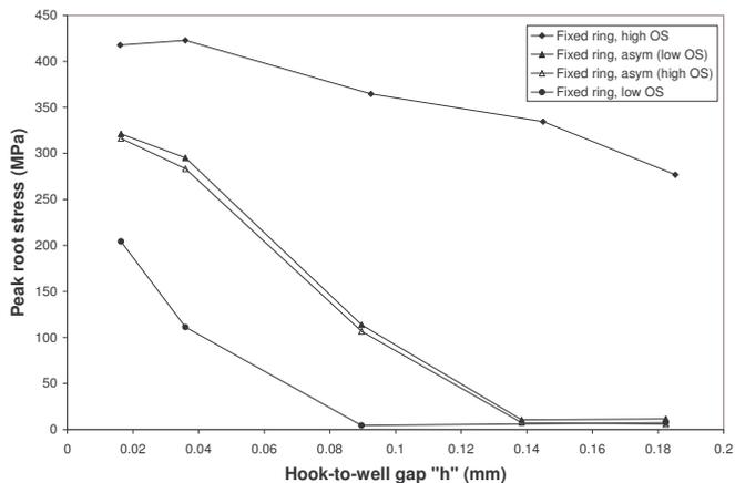
Figure 3: Effect of hook to well gap and position of attachment of outlet strut legs to valve ring on stresses at root of outlet strut for a rigidly supported valve.
